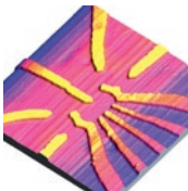
Pair of electrostatically-defined quantum dots
