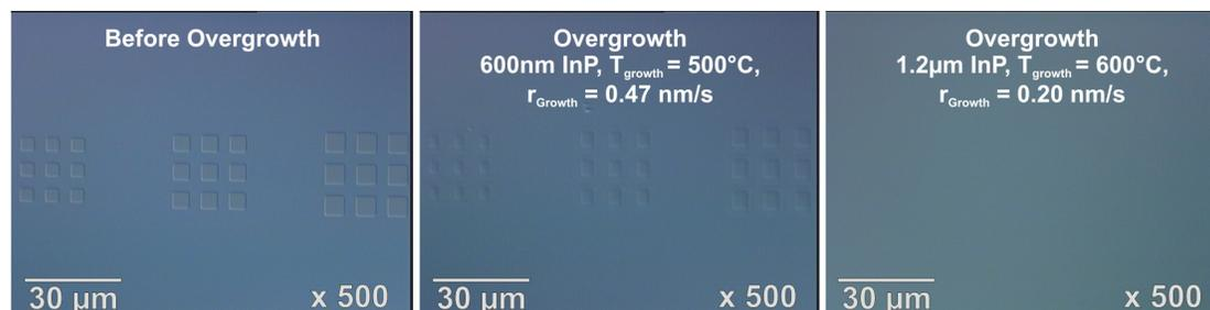
**Fig. 2:** The microscope images illustrate the planarization of the etched structures at 600°C, whereas at 500°C only an elongation in (01-1) direction could be observed
