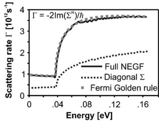
**Fig. 2** On-shell scattering rate of electrons by screened polar optical phonons in homogeneous GaAs at 300 K, resulting from full NEGF calculations (full line) and with purely on-site self-energies  $\Sigma$  (dotted line). The scattering rate obtained from the Fermi Golden rule is shown for comparison (grey dots)
