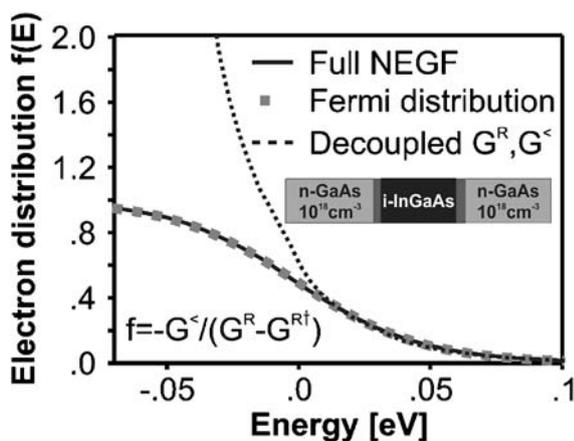
**Fig. 1** Equilibrium electron distribution of a 12 nm wide GaAs/ $\text{In}_{.14}\text{Ga}_{.86}\text{As}$  quantum well at 300 K calculated with fully self-consistent NEGF (full line) and with decoupled retarded and lesser Green’s functions (dashed). The zero of energy is the chemical potential. The full NEGF result faithfully yields the Fermi distribution (grey dots), in contrast to the decoupled model that violates the Pauli principle
