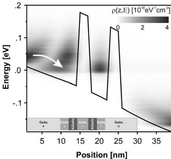
**Fig. 4** Conduction band profile of GaAs/Al<sub>3</sub>Ga<sub>7</sub>As resonant tunneling structure as described in the text, plotted at the resonant bias voltage of 200 mV. The energy resolved electron density is shown as contour plot. The arrow is meant to guide the eye and shows the trapping of electrons into the triangular quasi-bound state in front of the barriers
