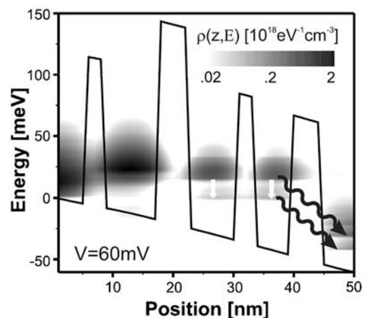
**Fig. 5** Conduction band profile of 50 nm GaAs/Al<sub>15</sub>Ga<sub>85</sub>As quantum cascade laser structure from Ref. [10] at a bias voltage of 60 mV and at 100 K. The energy resolved electron density is shown as contour plot. The arrows are only meant to guide the eye and show the calculated emission energies (white = photons, black = phonons)
