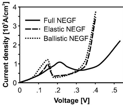
**Fig. 3** Calculated current density in the GaAs/Al<sub>3</sub>Ga<sub>7</sub>As resonant tunneling structure of Fig. 4 as a function of applied bias. The full NEGF calculations (full line) are compared with approximate models that invoke solely elastic scattering (dashed) or no incoherent scattering at all (dotted)
