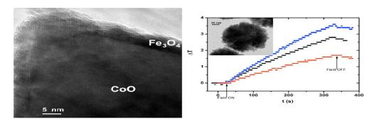
Figure 1. High resolution TEM image of a magnetic core-shell CoO-Fe3O4 nanoparticle and temperature kinetics of aqueous dispersions of colloidal clusters of manganese ferrite nanoparticles during the application of an alternating magnetic field.
